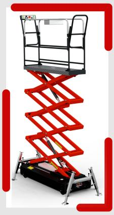
When the stabilizers are retracted, platform only rises to a height of 3m and allows moving on pipes so that it can be used as a care trolley, but when stabilizers are pulled out, the trolley automatically immobilizes the drive and there is a possibility of lifting up to 6m – this ensures a high level of employee safety.
